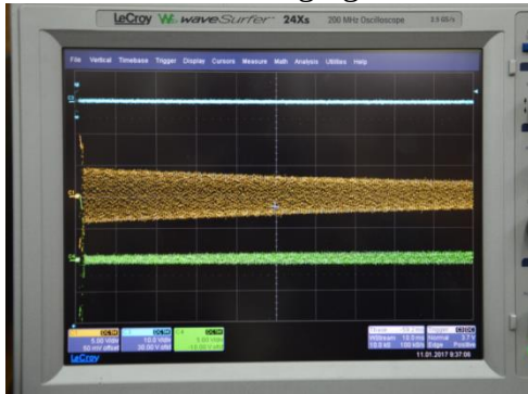
Fig. 13. Observation of swinging of the main channel only. There are oscillations in the quadrature channel appear too. We observe the transfer of energy from the main channel to the quadrature channel
