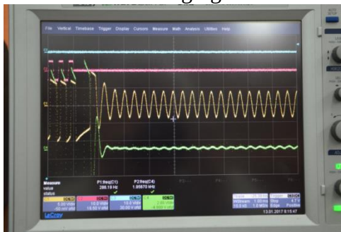
Fig.15. The oscillations in the main channel are excited. The oscillations in the quadrature channel are suppressed by the suppression pulses (red)
