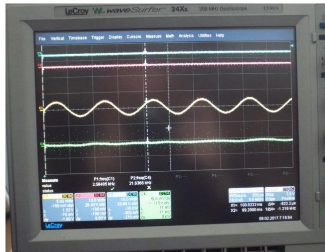
Fig. 18. The oscillogram after setting the suppression in the quadrature channel in the neighborhood of the time moment is 0.1 seconds. We observe almost complete suppression of the signal in the quadrature channel. The resonator is stationary
