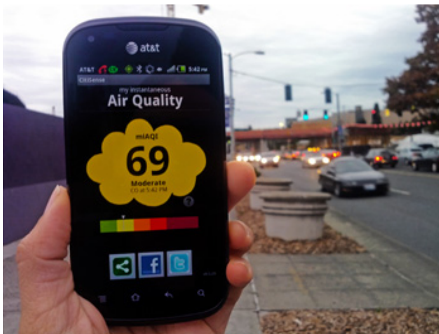
Figure 8: Prototyped “eco-phones” come equipped with air pollution sensors.
