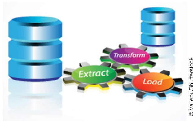
FIGURE 3.10 Data enter databases from transaction systems. Data of interest are extracted from databases, transformed to clean and standardize them, and then loaded into a data warehouse. These three processes are called ETL.
