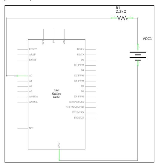
As seen in the previous schematic, the analog input pin labeled **A0** in the board's symbol, is connected to the positive terminal of the power source through the resistor. The negative terminal of the power source is connected to the ground.
