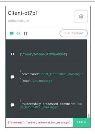
After you publish the previous message, you will see the following output in the SSH console for the Intel Galileo Gen 2 board. You will see the following text displayed at the bottom of the OLED matrix: 2nd message. The board also receives the successfully processed command message because it is subscribed to the channel in which the message has been published.
