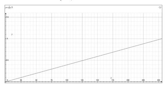
The equation for the previous graph is the following: y = x / 255 \* 5, specifically voltage = brightness / 255 \* 5. We can run the following code in our Python interpreter to see the output with all the voltages that will be generated for each brightness level from 0 to 255 inclusive.
