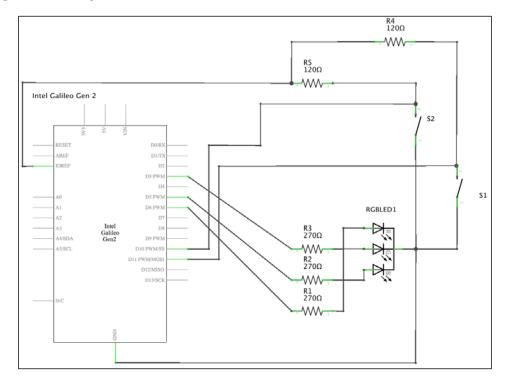
The GPIO pin labeled **D10 PWM/SS** in the board's symbol is connected to the **S2** pushbutton and the **R4** resistor is its pull-up resistor. The GPIO pin labeled **D11 PWM/MOSI** in the board's symbol is connected to the **S1** pushbutton and the **R5** resistor is its pull-up resistor. This way, GPIO pin number 10 will be low when the **S2** pushbutton is pressed and GPIO pin number 11 will be low when the **S1** pushbutton is pressed.
