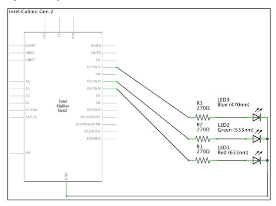
As seen in the previous schematic, three PWM capable GPIO pins labeled D3 PWM, D5 PWM and D6 PWM in the board's symbol is connected to a  $270\Omega$  resistor, wired to an LED's anode, and each LED's cathode is connected to ground.
