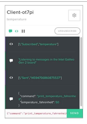
After you publish the previous message, you will see the following output in the SSH console for the Intel Galileo Gen 2 board. You will notice the servo's shaft rotates to 50 degrees.
