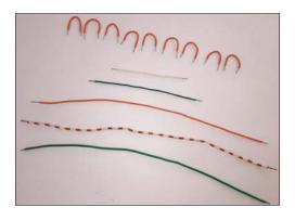
In case we don't want to spend time building our own jumper wires, we can buy prebuilt male to male solderless flexible breadboard jumper wires with tiny plugs attached to the wire ends.
