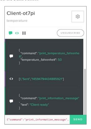
After you publish the previous message, you will see the following output in the SSH console for the Intel Galileo Gen 2 board. You will see the following text displayed at the bottom of the OLED matrix: Client ready.
