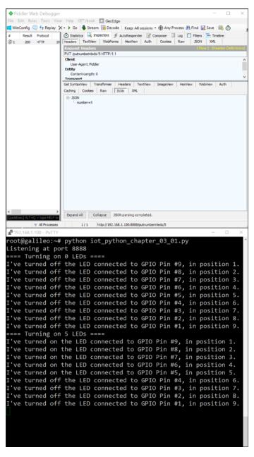
We can run the following HTTPie command in a computer or device to use the RESTful API to tell us how many LEDs are turned on.
