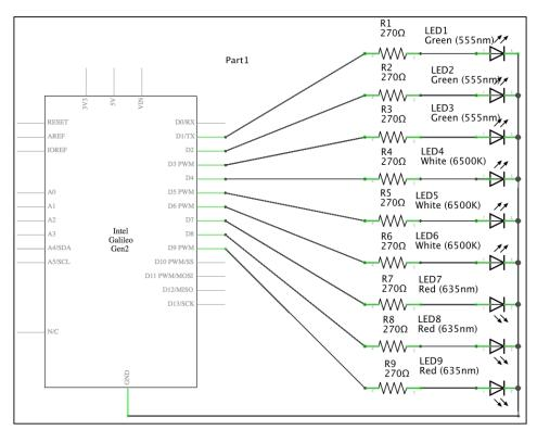
As seen in the previous schematic, each GPIO pin labeled from D1 to D9 in the board's symbol is connected to a  $270\Omega$  resistor, wired to an LED's anode, and each LED's cathode is connected to ground. This way, whenever we write a high (1) value to any of the GPIO pins, the board will put 5V on the pin and the LED will turn on. Whenever we write a low (0) value to any of the GPIO pins, the board will put 0V on the pin and the LED will turn off.
