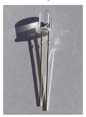
The LED in the picture is located in the same position than the LEDs are connected in the previously shown breadboard picture. Thus, we have to connect the shorter lead at the left and the larger lead at the right in the breadboard. The next picture shows the LED representation in the breadboard picture with its cathode and anode.
