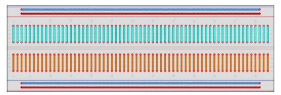
The breadboard provides two power lanes, bus strips or horizontal buses at the top and at the bottom of the board. These power lanes connect all the holes within the row. Each column has five row holes connected.
