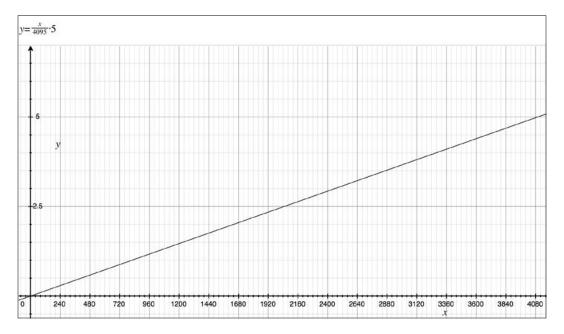
The equation for the previous graph is y = x / 4095 \* 5, specifically voltage\_value = analog\_pin\_read\_value / 4095 \* 5. We can run the following code in our Python interpreter to see the output with all the voltage values that can be generated with the formula for each raw value read from the analog pin from 0 to 4095 (inclusive).
