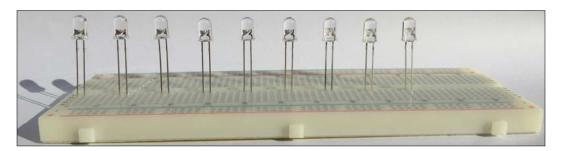
The following picture shows all the LEDs connected to the breadboard where you can check that the LEDs are connected as we have seen in the breadboard view for the Fritzing diagram.
