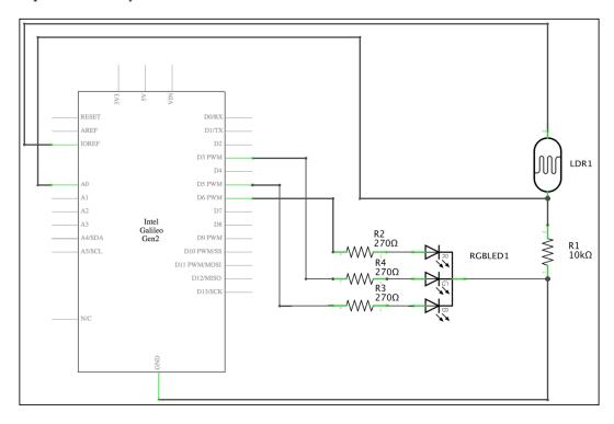
As seen in the previous schematic, three PWM capable GPIO pins labeled **D3 PWM**, **D5 PWM**, and **D6 PWM** in the board's symbol is connected to a  $270\Omega$  resistor, wired to an anode pin for each LED color, and the common cathode is connected to ground.
