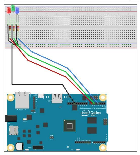
In this case, we wanted the three LEDs to be close to each other. This way, the three LEDs can project their light to a black surface and we can see how the intersection of the three colors generates a color that will be similar to a color selected in a color picker we will use later.
