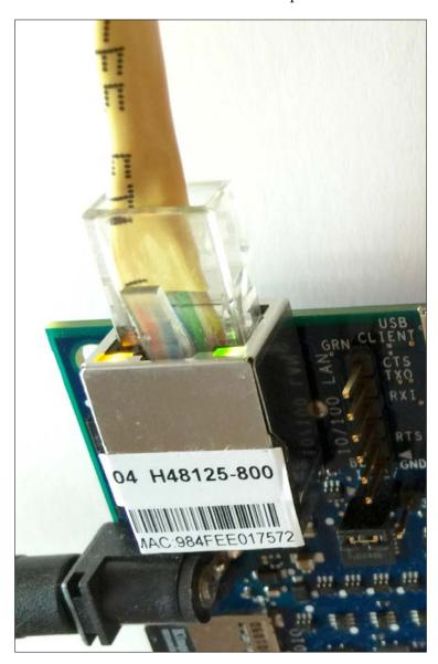
A six pin, 3.3V USB TTL UART header is located next to the Ethernet jack, specifically UART 1, the second UART port in the board. The six pin, 3.3V USB TTL UART header has the following labels on the right-hand side:
