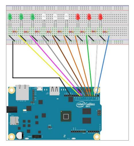
Now, whenever we want to turn on LED 1, we must write a high (1) value to GPIO pin number 9, whenever we want to turn on LED 2, we write a high (1) value to GPIO pin number 8, and so on. Because we changed the wirings, the schematic with the electronic components represented as symbols also changed. The following picture shows the new version of the schematic.
