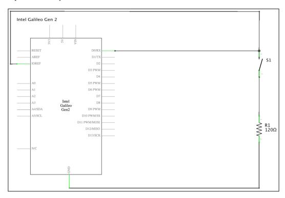
As seen in the previous schematic, in this case, the GPIO pin labeled **D0/RX** in the board's symbol is connected to the **S1** pushbutton and the **IOREF** pin. The other connector of the S1 pushbutton is wired to the  $120\Omega$  resistor and this resistor is wired to **GND** (ground).
