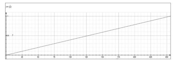
The equation for the previous graph is the following: y = x / 255, specifically value = brightness / 255. We can run the following code in our Python interpreter to see the output with all the values that will be written for each brightness level from 0 to 255 inclusive.
