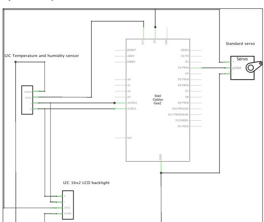
The following picture shows the schematic with the electronic components represented as symbols:
