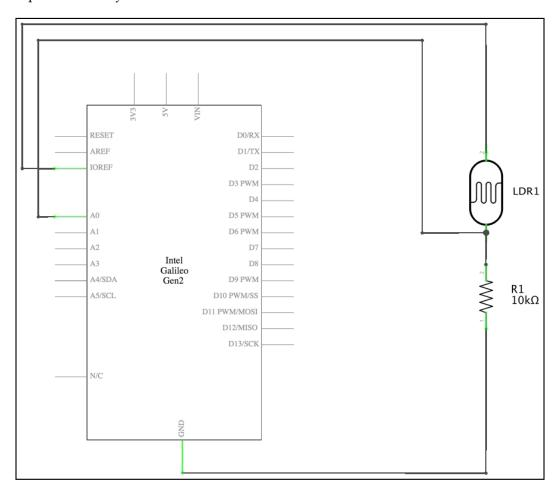
As seen in the previous schematic, the GPIO pin labeled A0 in the board's symbol is connected to the voltage divider built with the photoresistor named LDR1 and a  $10k\Omega$  resistor with 5% tolerance named R1. The LDR1 photoresistor is wired to the IOREF pin. We already know that the pin labeled IOREF provides us the IOREF voltage, that is, 5V in our actual configuration. The R1 resistor is wired to GND (ground).
