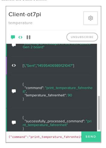
After you publish the previous message, you will see the following output in the SSH console for the Intel Galileo Gen 2 board. You will notice the servo's shaft rotates to 90 degrees. The board also receives the successfully processed command message because it is subscribed to the channel in which the message has been published.
