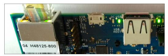
The following image shows the side view with all the connectors and jacks. From left to right, the USB 2.0 port, the micro USB connector, the UART header, and the Ethernet jack with the green (SPEED) and yellow (LINK) LEDs.
