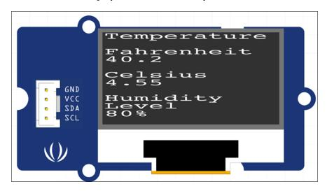
After we replace the LCD screen breakout board with the OLED module, we will have the following connections:
