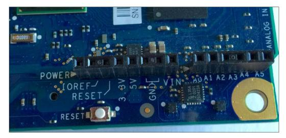
The board includes a jumper labeled **IOREF** that allows us to select between a 3.3V or 5V shield operation and provides voltage-level translation to all the I/O pins. Based on the jumper position, the board can work with either a 3.3V or 5V Arduino shield. By default, the **IOREF** jumper is set to the 5V position, and therefore, the initial setting allows us to work with 5V shields. The following screenshot shows the **IOREF** jumper set to the 5V position.
