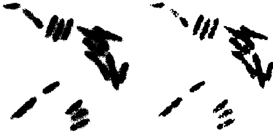
Figure 6.8: (Left) Binary image of bacteria (in the original microscope image, the bacteria were blue due to their fluorescence); (right) cleaner image resulting from changing black pixels that had one or more white neighbors to white. Original image courtesy of Frank Dazzo.
