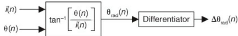
Figure 13-60 Frequency demodulator using an arctangent function.
