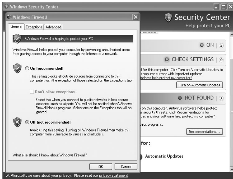
Figure 1-33: Turning off the Windows firewall
