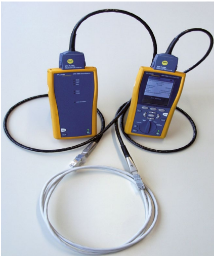
Test for a short permanent link (PL2) using the DTX 1800 Cable Analyzer
