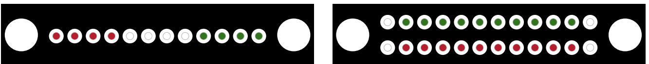
12-fiber (left) and 24-fiber (right) MPO connectors. Color highlighting shows fibers for sending (red) and receiving (green).
