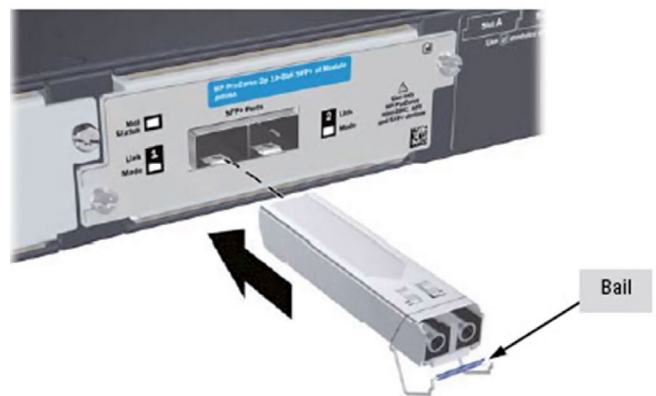
SFP / SFP+: 8.5 x 13.4 x 56.5mm [Image: Cisco]
