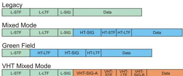
Figure 4) WLAN Frame Format
