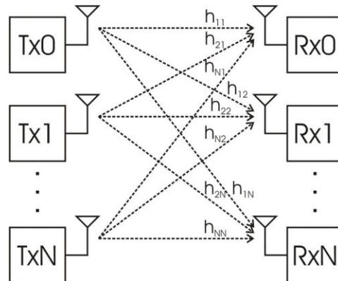
Figure 2) SDM Channel Using MIMO Topology
