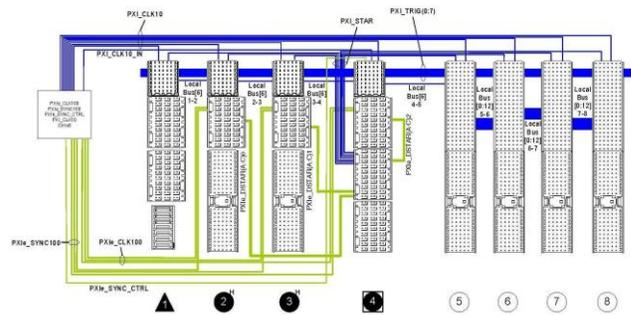
Figure 11) PXIe Backplane Trigger & Clock Routing
