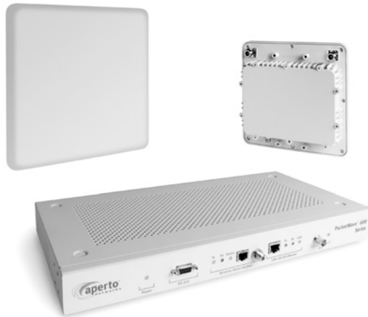
Figure 13-3: A Base Station Transmitter (Courtesy of Aperto Networks Inc.)
