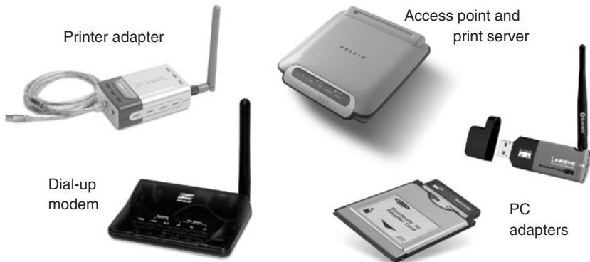
Figure 3-20: A Variety of Bluetooth Devices (courtesy of Belkin Corporation, D-Link (Europe) Ltd., Linksys (a division of Cisco Systems Inc.) and Zoom Technologies, Inc.)
