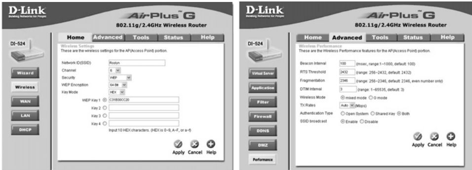
Figure 7-4: Typical Access Point Configuration Screens
