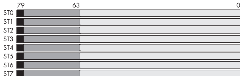
Figure 6-1: FPU floating-point register stack
