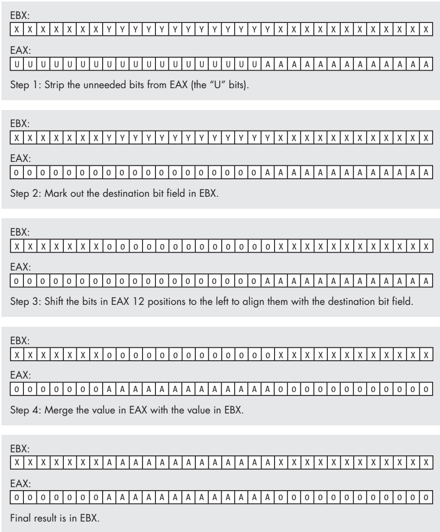
Figure 10-2: Inserting bits 0..12 of EAX into bits 12..24 of EBX
